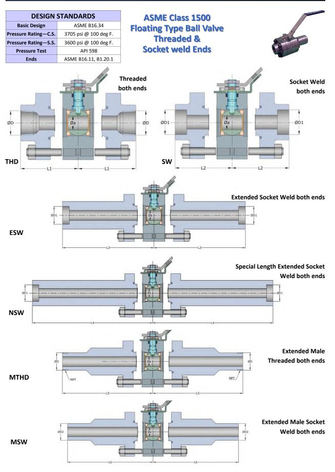
All end configurations are integral components—no welding is used.
